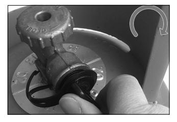
3. Check the bullnose connection on the regulator for any visible damage before connecting to the cylinder.
